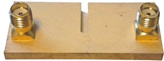
FIGURE 24. Isometric view of the fabricated fourth-order filter with four transmission zeros located above the passband.
