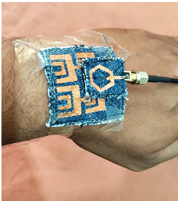
FIGURE 11. Antenna placed on human wrist.
