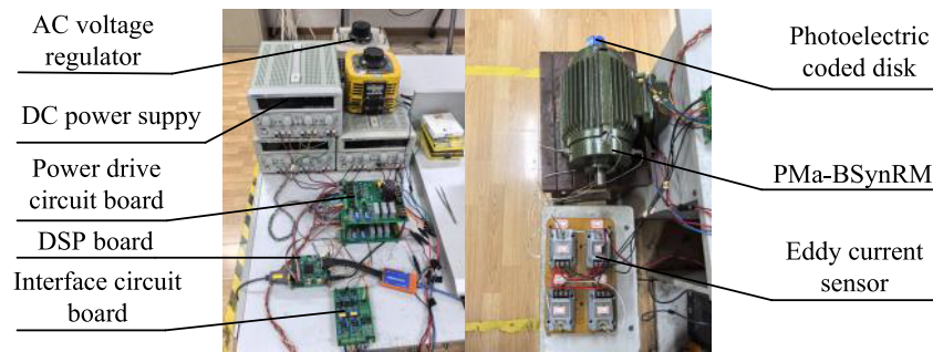
FIGURE 17. The experimental platform of PMa-BSynRM.
