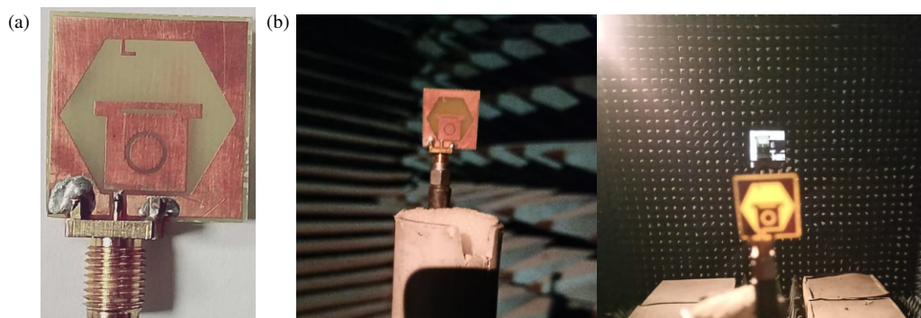
FIGURE 8. Measurement setup and antenna prototype: (a) Fabricated antenna. (b) Anechoic chamber configuration.
