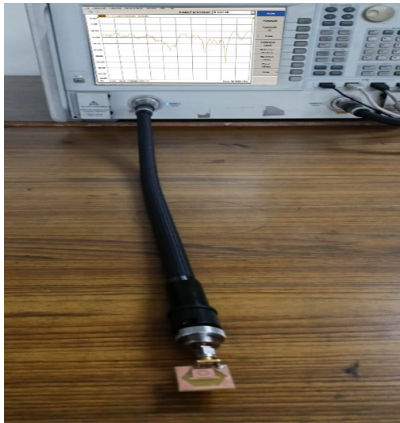
FIGURE 10. Antenna |S_{11}| VNA measurement setup.
