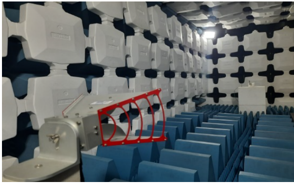
FIGURE 14. Antenna radiation pattern and gain measurement in an anechoic chamber.
