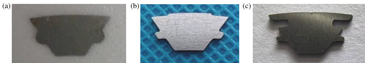
FIGURE 17. Stamping sheet for rotor. (a) Conventional rotor. (b) Surface auxiliary slots rotor. (c) Internal auxiliary slots rotor.
