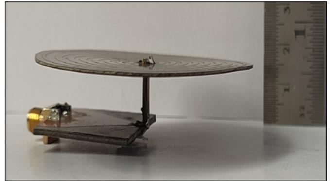
FIGURE 13. Fabricated modified balun with spiral antenna.
