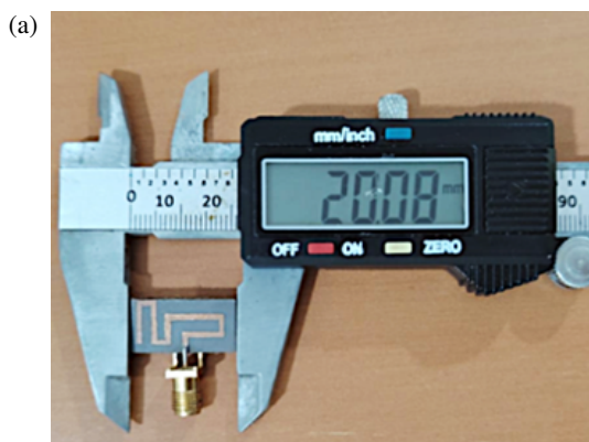
FIGURE 5. Images of the fabricated antenna prototype: (a) top view and (b) bottom view.
