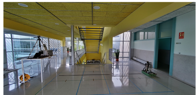
FIGURE 2. Measurement environment with reference grid on the floor. Tx antenna on the right, Rx on the left.
