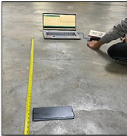
FIGURE 27. The distance between the hardware and mobile application is 1 m.
