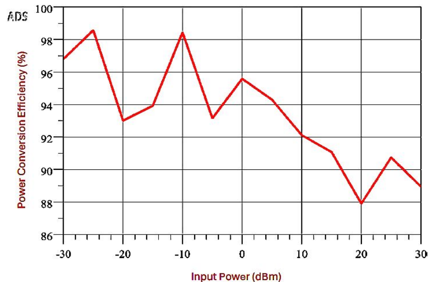
FIGURE 13. Rectenna simulated power conversion efficiency at 2.45 GHz vs. different input power values.
