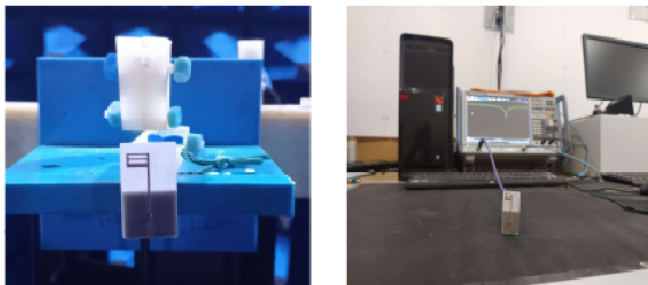
FIGURE 14. Measurement of antenna in an anechoic chamber.
