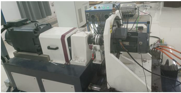
FIGURE 15. VLF-RSPM radial electromagnetic force wave test platform.
