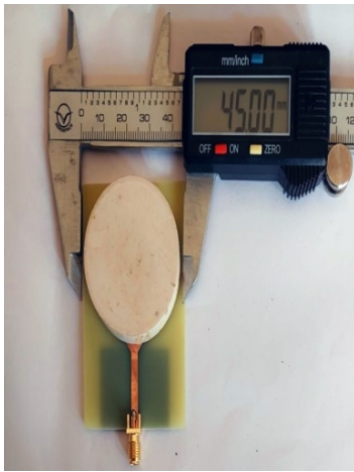
FIGURE 8. Proposed assembled antenna prototype topmost view.
