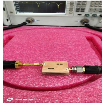
FIGURE 4. Fabricated prototype and measurement evidence: Top view, bottom/DGS view, anechoic chamber arrangement, and VNA setup.
