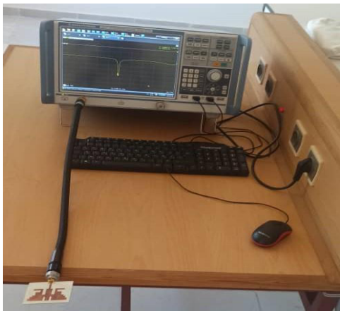
FIGURE 8. Reflection coefficient setup measurement of the antenna 2 GHz in free space.
