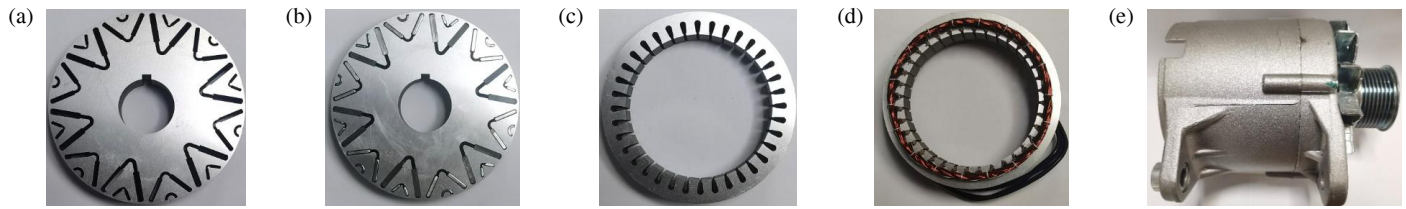
FIGURE 21. Generator prototype. (a) Rotor core, (b) rotor, (c) stator core, (d) stator, and (e) prototype.
