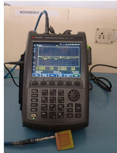
FIGURE 9. Keysight VNA measurement setup.
