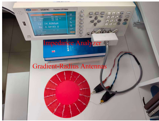
FIGURE 6. Impedance measurement experiment.
