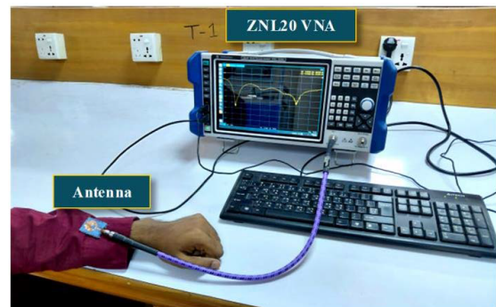
FIGURE 12. Experimental setup for S_{11} measurement.
