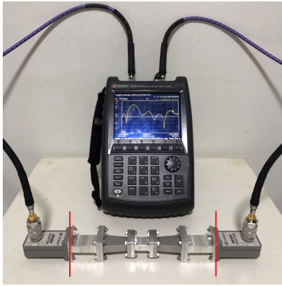
FIGURE 7. VNA measurement setup of the waveguide component. The red line indicates the calibration plane of the WR90 calibration kit.
