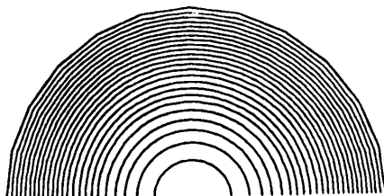
Figure 5.25a Real part of eddy-current profile in cross section of round bar without crack.
