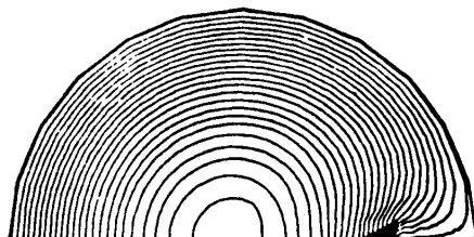
Figure 5.25b Real part of eddy-current profile in cross section of round bar with crack.
