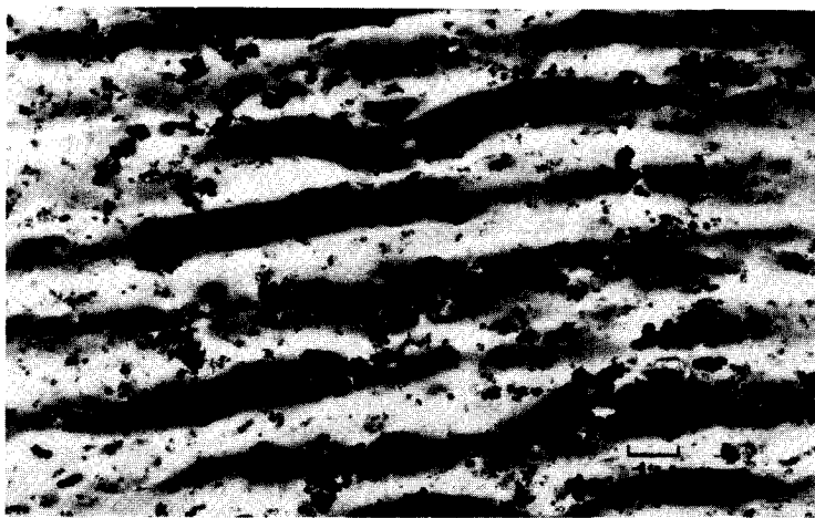
Figure 7.6 TEM of Poly(carbonate)-Carbon black (acetylene black) composite ( \phi \approx 6.4\% , magnification 7500).
