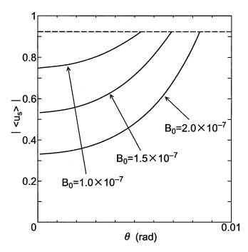
Figure 9. Bistatic scattering characteristics of the coherent wave under the condition of  $B_o l_o$  constant, where the broken line shows that the effect of double passing is not included in  $|\langle u_s \rangle|$ .
