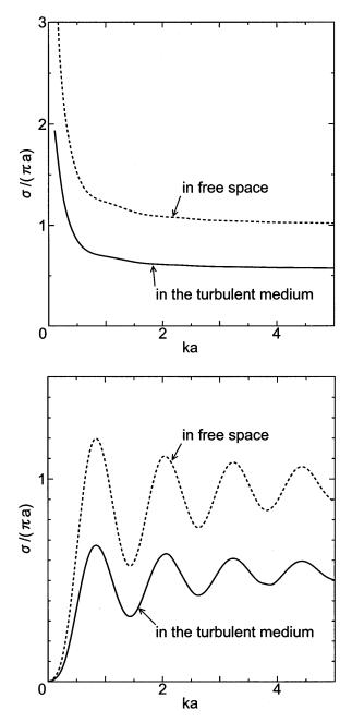
Figure 8. Backscattering cross-sections vs. cylinder size, calculated from the coherent scattered waves. (a) E-wave incidence case. (b) H-wave incidence case.
