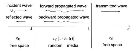
Figure 5. Geometry of the propagation problem in a random medium.
