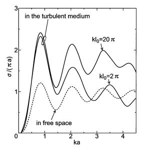
Figure 17. The average backscattering cross-section in the case of Hwave incidence, where the coherence length of the incident wave is shown in Figure 18.
