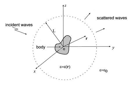
Figure 1. Geometry of the problem of wave scattering from a conducting body in an inhomogeneous medium.
