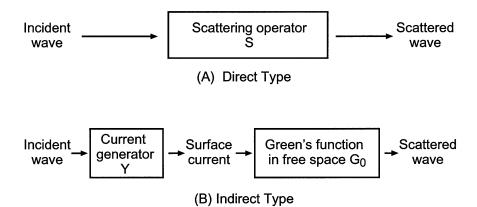
Figure A-1. Schematic diagram for solving the scattering problem where a conducting body is in free space.
