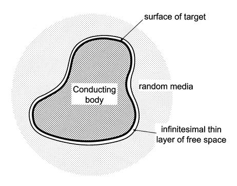
Figure 2. A model of the boundary between a body and a medium.
