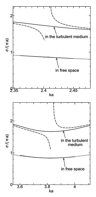
Figure 15. The average backscattering cross-sections about the internal resonance frequencies in the case of H-wave incidence. (a) In the neighborhood of the first zero point of  $J_o(ka_o) : ka_o = 2.40482 \cdots$  (b) In the neighborhood of the second zero point of  $J_1(ka_o) : ka_o = 3.83171 \cdots$ .
