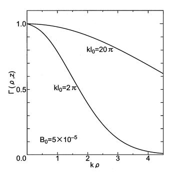
Figure 18. The degree of spatial coherence of incident waves about the cylinder. This figure shows that the coherence length of the incident wave becomes short, compared with Figure 10.
