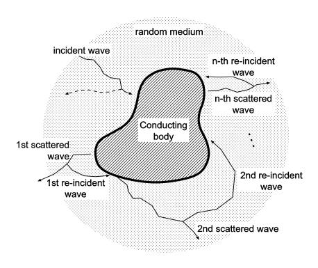
Figure 3. A model of scattering.
