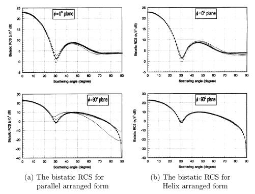
**Figure 6.** The circle, square, triangle, and cross signals denote the results for the threshold  $\varepsilon = 0, 0.01, 0.05, 0.1$ . The Bistatic RCS on  $\phi = 0^{\circ}$  and  $\phi = 90^{\circ}$  for the two kind of arranged forms.
