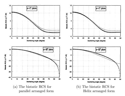
**Figure 4.** The circle, square, triangle, and cross signals denote the results for the threshold  $\varepsilon = 0, 0.01, 0.05, 0.1$ . The Bistatic RCS on  $\phi = 0^{\circ}$  and  $\phi = 90^{\circ}$  for the two kind of arranged forms.
