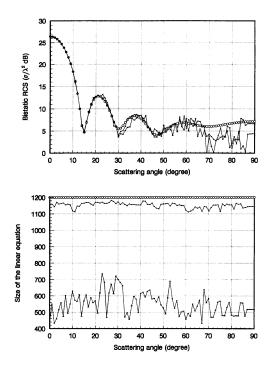
**Figure 8.** The circle, triangle, and cross signals denote the results for the threshold  $\varepsilon = 0, 0.01, 0.05$ . The monostatic RCS and size of the linear equation for H-polarized plane wave.
