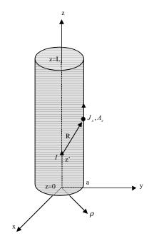
Figure 3. Wire structure in the cylindrical coordinate system.
