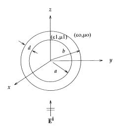
Figure 1. Geometry of the coated sphere.
