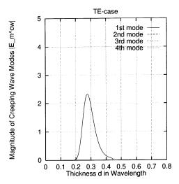
**Figure 8.** The magnitude of creeping wave modes from the attenuation constant (Fig. 5) and the diffraction coefficient (Fig. 6): TE-case. The first mode of the creeping wave is very significant when  $d = 0.28\lambda_o$  and the other modes are negligible when  $d = 0. \sim 0.8\lambda_o$ .
