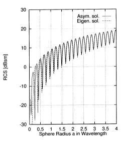
**Figure 2.** RCS from a coated sphere with the coating material  $\epsilon_r = (2.5, -0.2)$  and  $\mu_r = (1.6, -0.1)$  and the thickness of coating  $d = 0.05\lambda_o$ .
