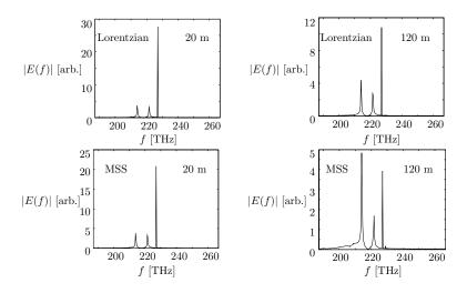
Figure 7. Raman pumping of probes spaced 5.5 and 13 THz apart from the pump. Raman gain spectrum modeled by a single Lorentzian resp. by the modified Sellmeier series (MSS) according to equation (17) and Tab. 1.
