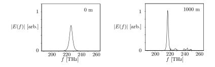
Figure 6. Spectra showing soliton self-frequency shifting.
