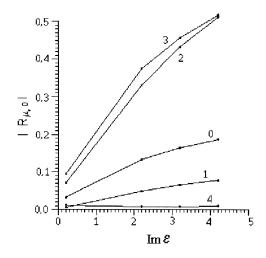
**Figure 3.** The dependence of the absolute value  $|R_{\mu,0}|$  of the Bloch reflection coefficient on the imaginary partx  $\Im \epsilon$  of the lower half-space dielectric permittivity for modes  $\mu = 0, \pm 1, \pm 2, \pm 3, \pm 4$  and under conditions  $\Re \epsilon = 1.50$ ,  $\alpha = 0$ ,  $h/\lambda = 0.75$ ,  $\kappa = \lambda/\Lambda = 0.3$ .
