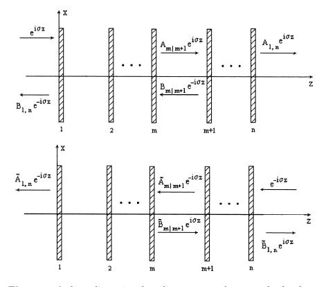
Figure 1. A three-dimensional medium presented as a stack of n layers with splits between them. In the top and bottom pictures the wave be incident upon the 1 st and the n's layer of the stack, respectively.
