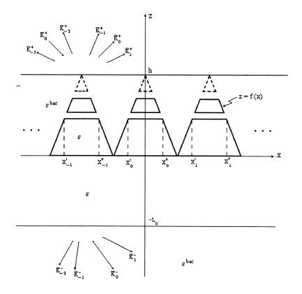
**Figure 2.** A periodic one-dimensional interface of two dielectric half-spaces with the dielectric permittivities  $\varepsilon^{bac}$  (upper half-space) and  $\varepsilon$  (lower half-space). An auxiliary truncated interface is presented in the form of a thin slice separated by a split from the rest truncated interface. The wave vectors of upgoing reflected and downcoming transmitted Bloch waves are depicted.
