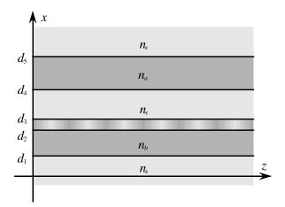
Figure 1. Geometry of the grating-assisted directional coupler.
