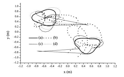
**Figure 9.** Inversion results of example 3 with noise-free data (a) true profile (b) initial guess (c) starting point for NKM and (d) inversion result after one Newton-Kantorivitch iteration. The final result is exactly the same as the true profile.
