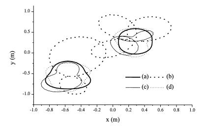
**Figure 8.** Inversion results of example 2 with noise-free data (a) true profile (b) initial guess (c) starting point for NKM and (d) inversion result after one Newton-Kantorivitch iteration. The final result is exactly the same as the true profile.
