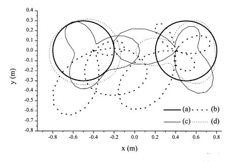
**Figure 4.** Inversion results of example 1 with noise-free data (a) true profile (b) initial guess (c) starting point for NKM and (d) inversion result after one Newton-Kantorivitch iteration. The final result is exactly the same as the true profile.
