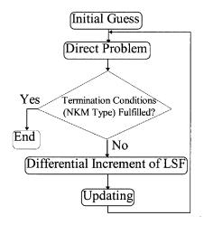
**Figure 3.** Flow chart of NKM for microwave imaging of two parallel perfectly conducting cylinders.
