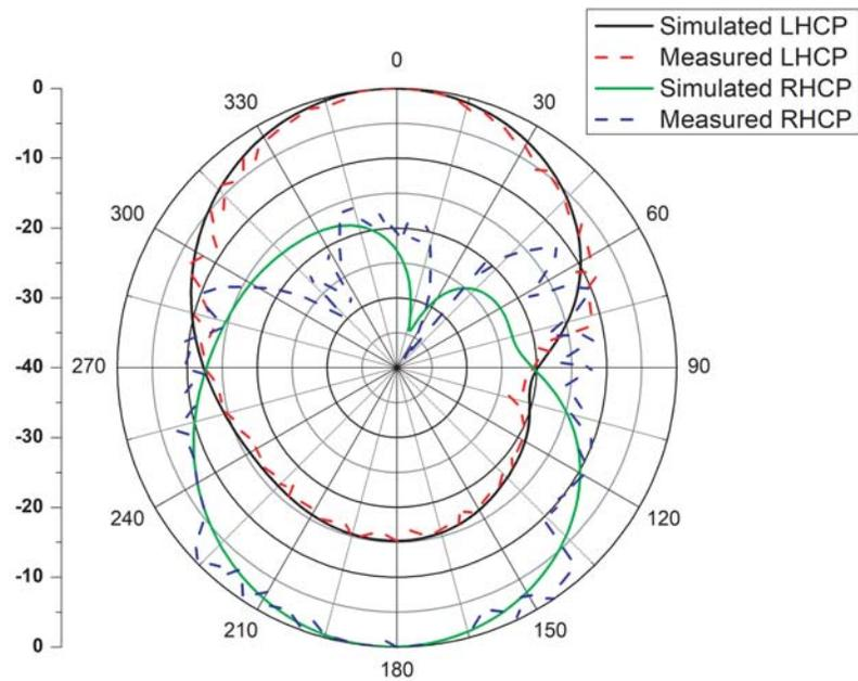
**Figure 12.** Measured and simulated radiation patterns at 3.5 GHz.
