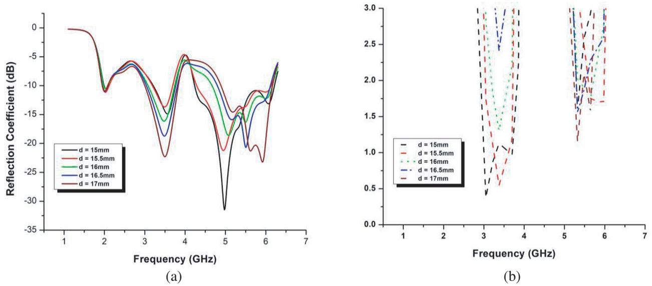
**Figure 6.** Effect of  $d$  on (a) reflection coefficient and (b) axial ratio.
