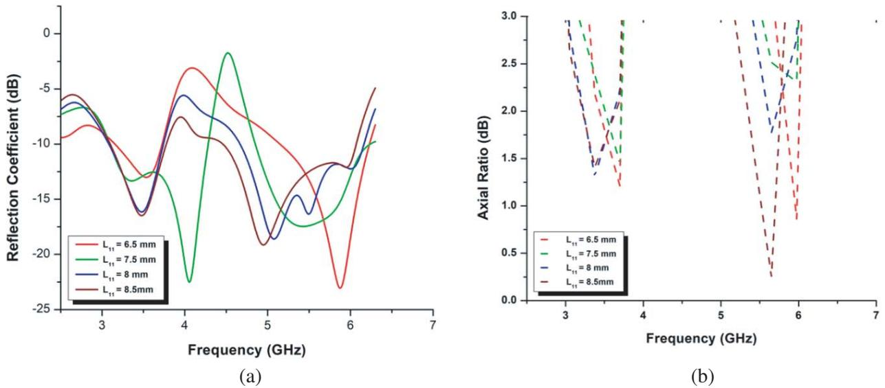
**Figure 7.** Effect of length  $L_{11}$  on (a) reflection coefficient and (b) axial ratio.
