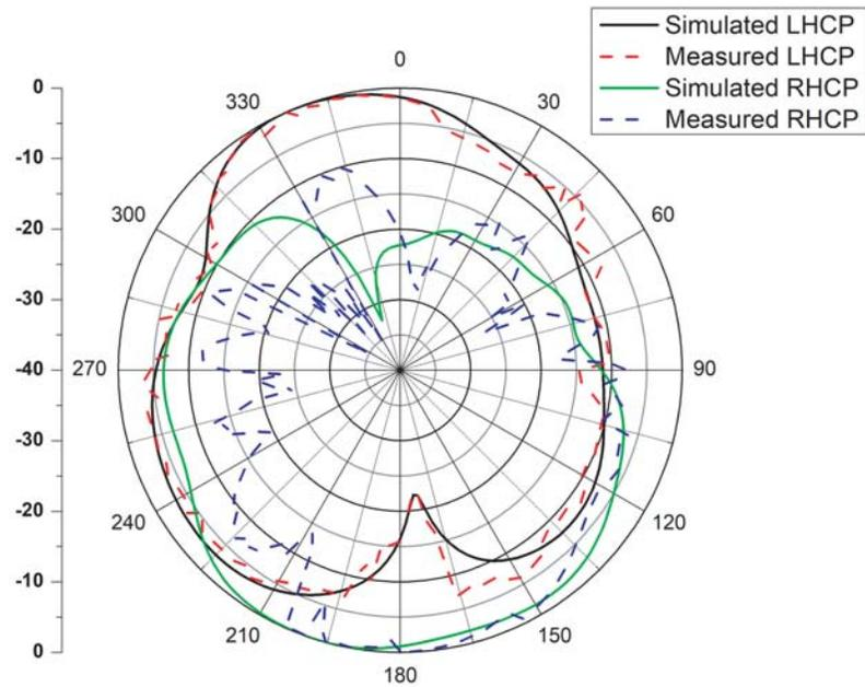
**Figure 13.** Measured and simulated radiation patterns at 5.5 GHz.
