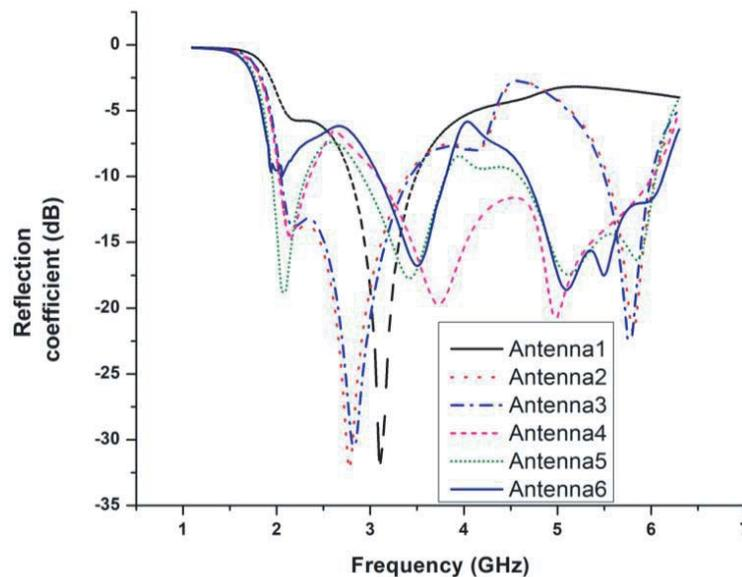
**Figure 4.** Simulated reflection coefficient for antenna I-V.
