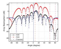
Figure 3. Comparison of the beampatterns of SCB, RCB and proposed method ( $\Delta \theta = 6^{\circ}$ , SNR = 30 dB,  $INR_1 = INR_2 = 20 \text{ dB}$ ).
