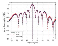
Figure 2. Comparison of the beampatterns of SCB, RCB and proposed method ( $\Delta \theta = 0$ , SNR = 10 dB,  $INR_1 = INR_2 = 20 \text{ dB}$ ).
