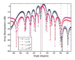
Figure 1. Comparison of the beampatterns of different diagonal loading levels  $(\Delta \theta = 4^{\circ})$ .
