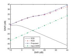
Figure 4. Comparison of the SINRs of SCB, RCB and proposed method ( $\Delta \theta = 3^{\circ}$ ,  $INR_1 = INR_2 = 20 \text{ dB}$ ).
