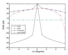
Figure 5. Comparison of the SINRs of SCB, RCB and proposed method (SNR = 30 dB,  $INR_1 = INR_2 = 20 \text{ dB}$ ).
