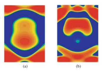
Figure 8. Field distribution at aperture of quasi TEM horn. (a) 3 GHz. (b) 6 GHz.
