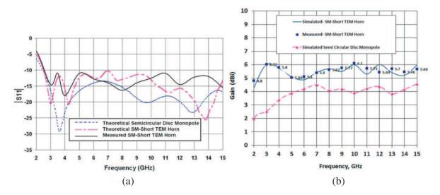
**Figure 4.**  $|S_{11}|$  of the CPW-fed disc monopole antenna with and without the short horn. (b) Comparison of the measured peak gain of the CPW-fed disc monopole antenna, with and without the short horn.
