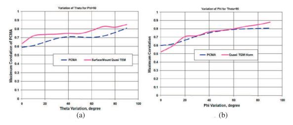
Figure 6. Pulse correlation of the new antenna and the reference semicircular disc monopole antenna, where theta is varying from Y to Z in yz-plane and phi is variation from X to Z in xz-plane.
