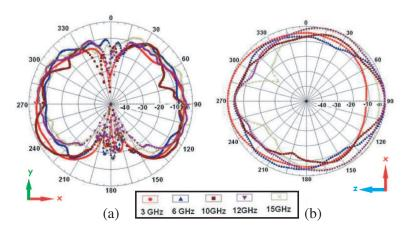
Figure 5. Measured radiation patterns. (a) X-Y plane. (b) X-Z plane.
