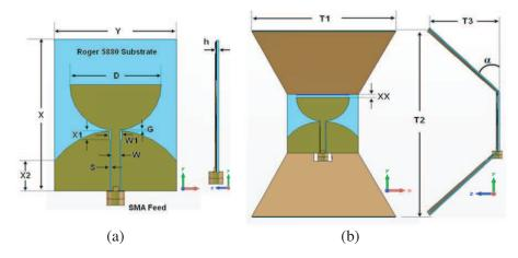
**Figure 1.** (a) CPW-fed semicircular disc monopole antenna. (b) CPW-fed semicircular disc monopole antenna with the printed surface- mounted short two-plate horn.
