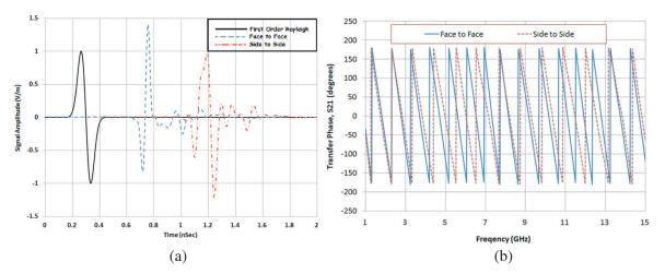
**Figure 7.** (a) Pulse performance of antenna. (b)Transmission phase of the new antenna for face to face and side to side arrangements.
